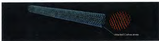
Fig. 1. Model of the molecular dynamic simulations. A single-wall carbon nanotube is placed on a substrate and a nanoparticle collides along the axial direction.
